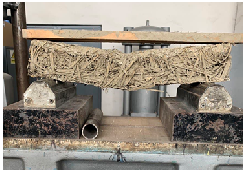
Fig.7. Determination of residual deformation from bending strength testing
