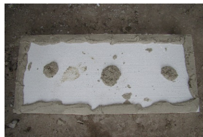
Fig. 2. Method to apply the adhesive mortar on polystyrene tiles
