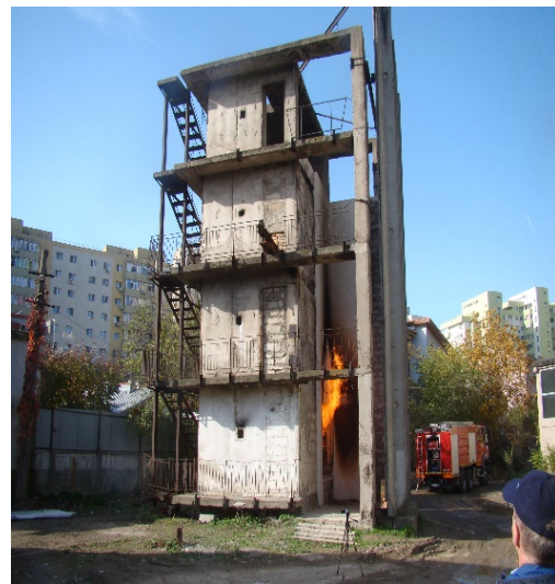
Fig. 7. Large scale fire testing of ETICS system
