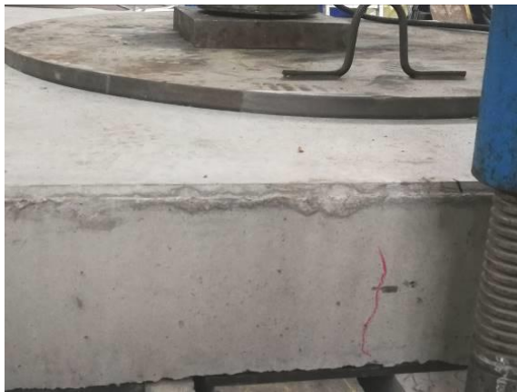
Fig. 8. Cover plate element cracking mode – 180 x 180 x 20 cm (B x L x h)
