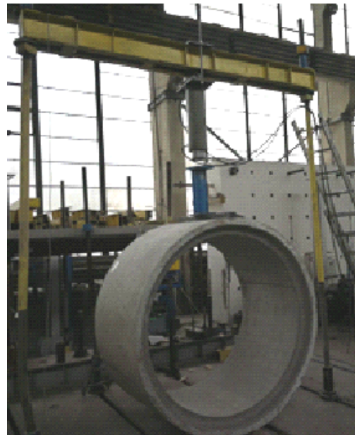
Fig. 1. Manhole straight element with DN160, during testing
