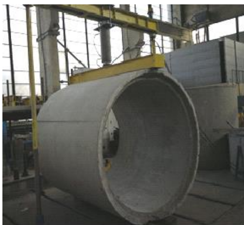
Fig. 3. Manhole straight element with DN200, during testing
