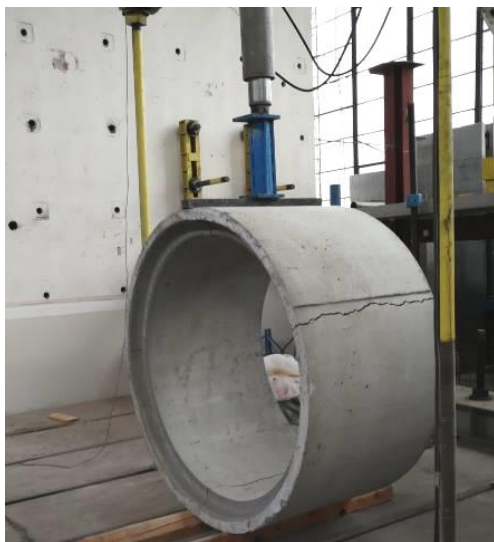
Fig. 2. Manhole straight element with DN160, after cracking, at failure
