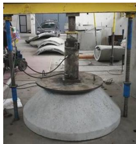
Fig. 5. Manhole element with DN160, during testing
