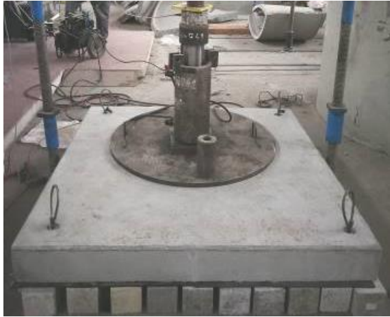
Fig. 7. Manhole cover plate type element, 180 x 180 x 20 cm (B x L x h), during testing
