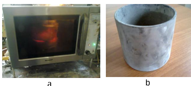
Fig. 1. The experimental microwave equipment (a – microwave oven; b – ceramic tube)
