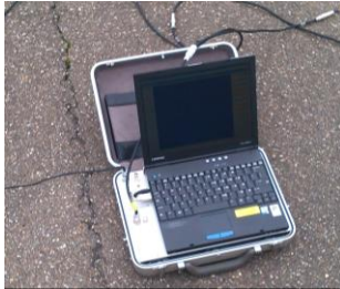
Fig. 17. Cross GEODAS acquisition station
