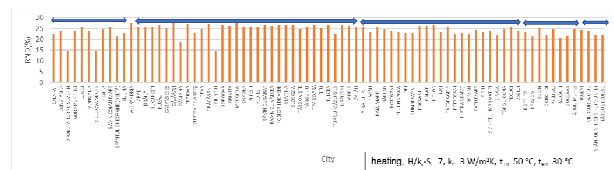
Fig. 2. Efficiency computed for heating, H/k_c \cdot S_c=7 , k_c=3 \text{ W/m}^2\text{K} , t_0=50 \text{ }^\circ\text{C} , t_{R0}=30 \text{ }^\circ\text{C}
