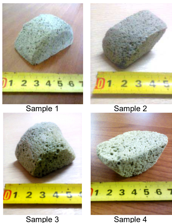
Fig. 2. Pictures of the foam glass gravel samples
