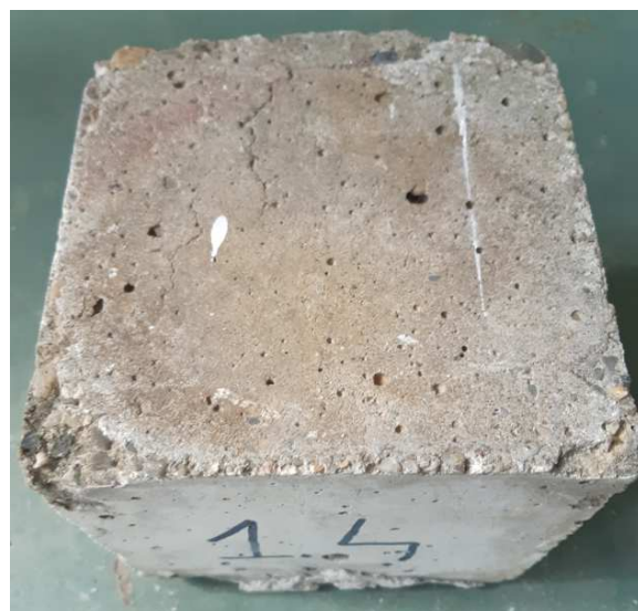
Fig. 6. Example of porous and surface cracks
