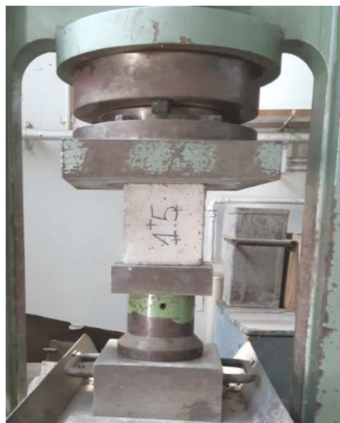
Fig. 11. Concrete cube ready for the rebound hammer test
