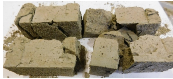
Fig. 7. Aspect of samples of mortar without wool after bending and compression
