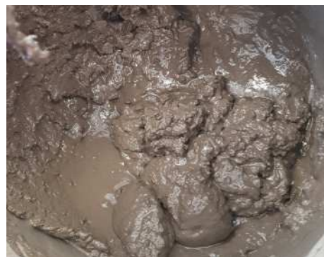
Fig.3. Fresh geopolymer paste
