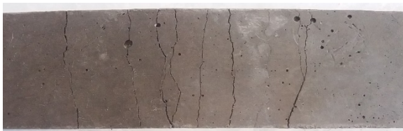
Fig. 2. Typical steady-state type of multiple cracks developed in ECC coupon specimen
