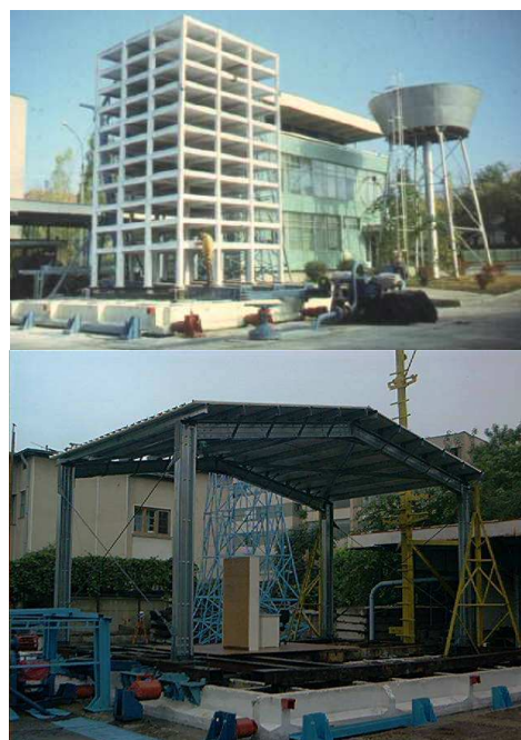
Fig. 1. Tests on seismic simulator (140 t) URBAN-INCERC, Iasi Branch (Diaconu, 2006)
