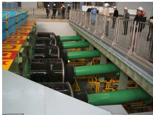
Fig. 4b. E-Defense NIED shaking table, Miki Town, Japan - the powerful actuators
