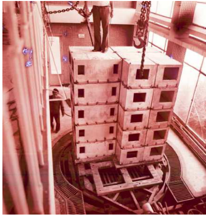
Fig. 2. Building of large panels on seismic simulator (shaking table of 15 t) URBAN-INCERC, Iasi Branch (Diaconu, 2006)
