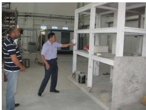
Fig. 6. Models of buildings in preparation for testing on shaking table/seismic simulator at China Academy of Building Research (RISKSOLVE PROJECT, 2013)
