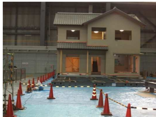
Fig. 4a. Natural scale house model on E-Defense NIED shaking table, Miki Town, Japan
