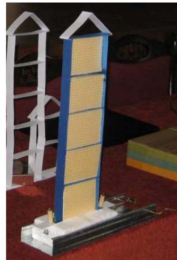
Fig. 12. Seismic mini-simulator "Crank-type"
