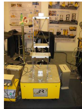
Fig. 9a. BUILDING TEST EXPO, Brussels, Belgium, 2014. Educational shaking table – seismic simulator for small building models
