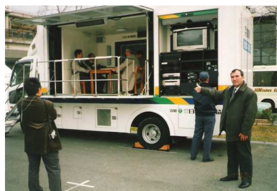
Fig. 7. Mobile seismic simulator available during WCDRR, Kobe, Japan, 2005. Persons on the platform are subjected to a seismic motion in successive steps
