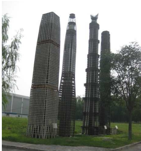
Fig. 5. Models of super-high buildings at scale 1:40, after testing at China Academy of Building Research, Platform Yanjiao (RISKSOLVE Project, 2013)
