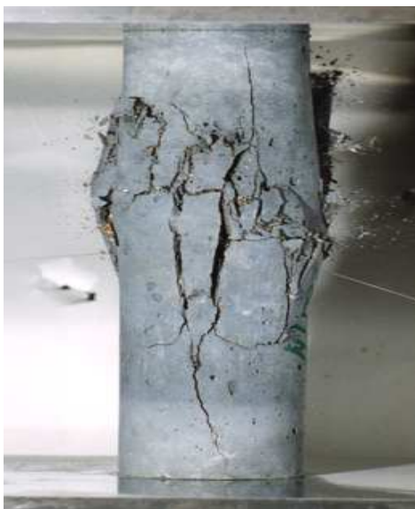
Fig. 1. Compressive failure of an UHPC cylindrical sample [8]
