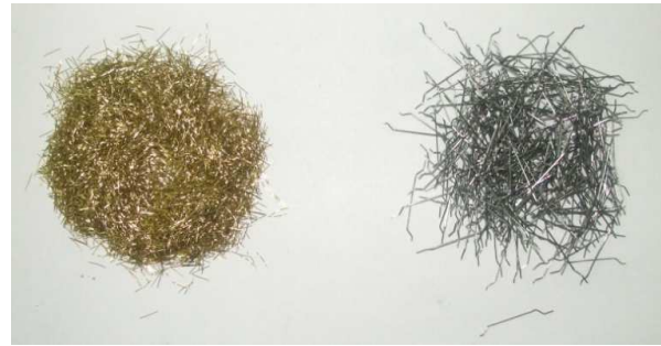
Fig. 5. Long (left) and short (right) steel-fiber reinforcement
