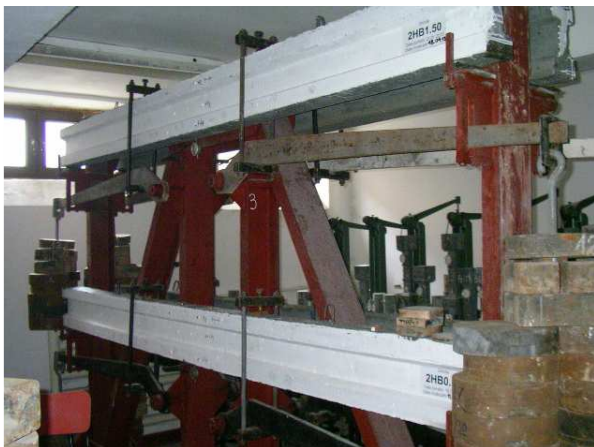
Fig. 7. UHPC beams subjected to long-term bending
