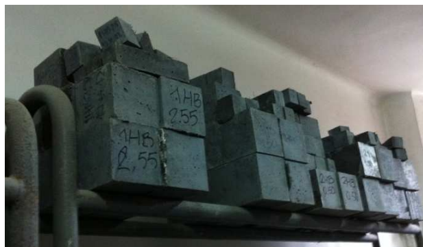
Fig. 4. UHPC samples kept in the climate chamber
