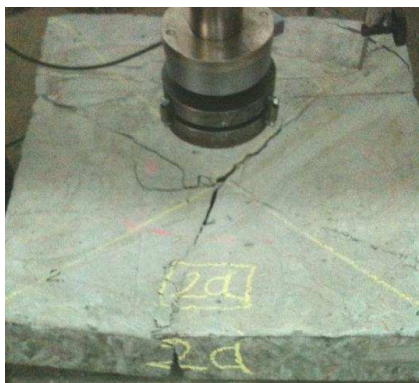
Fig. 13. Failure mode. Slab with 5 kg/m 3 PP fibers
