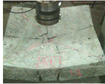
Fig. 14. Failure mode – Slab with 4 kg/m 3 PP fibers
