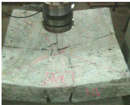
Fig. 12. Failure mode. Slab with 6 kg/m 3 PP fibers
