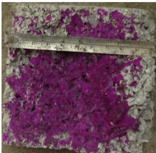
Fig. 13. Measuring the depth of carbonation
