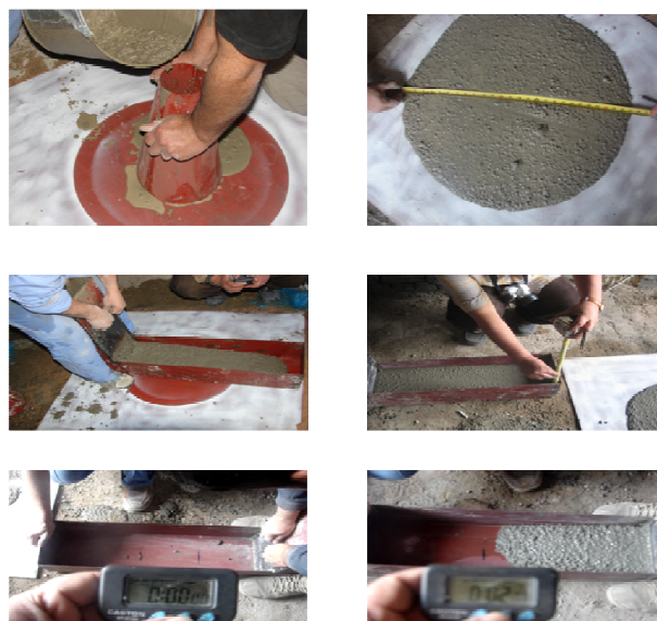
Fig. 2. Schematics of experimental tests for fresh properties of SCC
