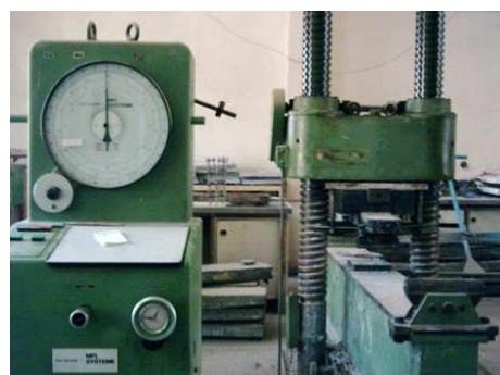
Fig.3. Universal testing machine used to test the beams
