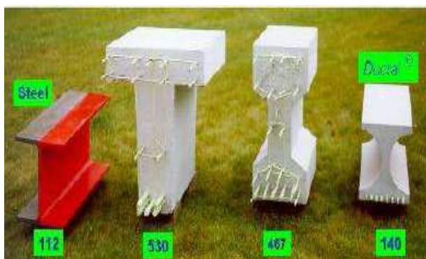
Fig. 2. Concrete and metal sections at equal load carrying capacity [7]
