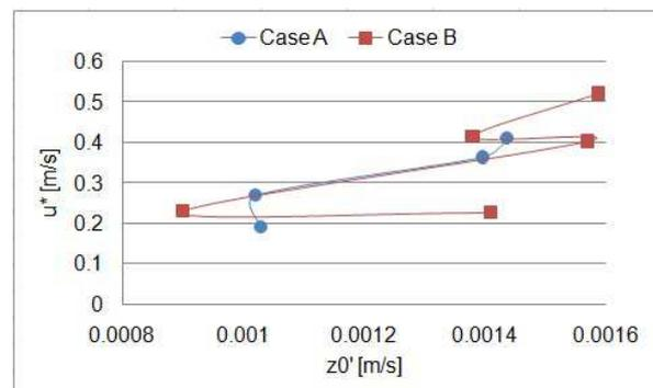
**Fig. 8.** Friction speed  $u^*$  depending on the roughness length  $z_0'$
