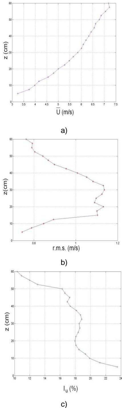
**Fig. 2.** Characteristics of the wind speed profile in the wind tunnel (urban exposure roughness):
