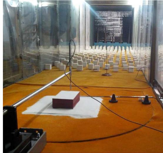
**Fig. 3.** The model placed in the tunnel and the three hot wire probes that measure the wind speeds,  $v_0$ ,  $v_1$  and  $v_2$
