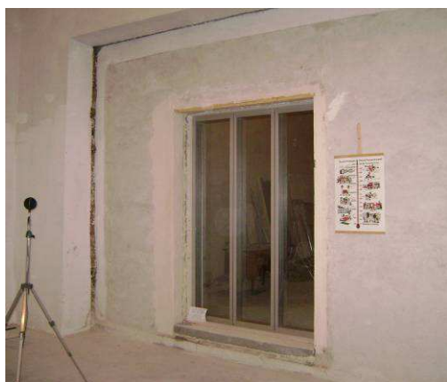
Fig. 7. Detail of the positioning of the partition wall system DIVIDO twinglass type (4-83-6), in the airborne sound insulation stand
