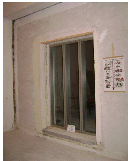
Fig. 8. Detail of the positioning of the partition wall system DIVIDO twinglass type (6-81-3.1.3), in the airborne sound insulation stand
