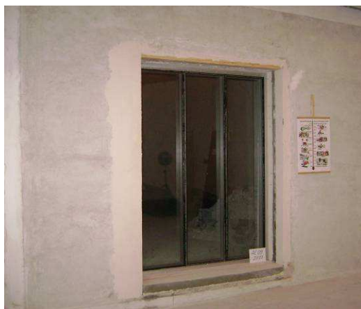
Fig. 4. Detail of the positioning of the partition wall system DUO glass type (6-85-8) in the airborne sound insulation stand
