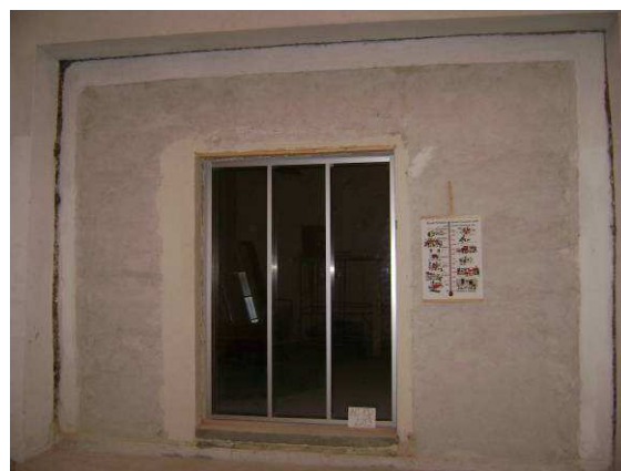
Fig. 9. Detail of the positioning of the partition wall system MODULO type (6-86-6), in the airborne sound insulation stand
