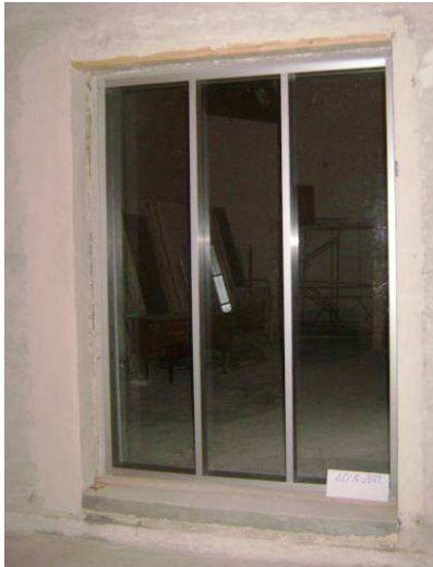
Fig. 10. Detail of the positioning of the partition wall system MODULO type (4-88-6), in the airborne sound insulation stand
