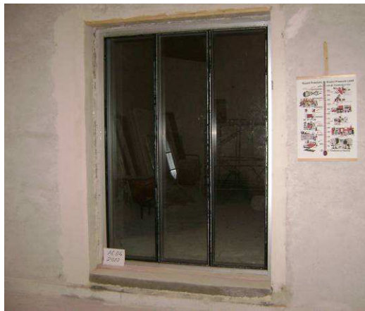
Fig. 3. Detail of the positioning of the partition wall system DUO glass type (6-87-6) in the airborne sound insulation stand
