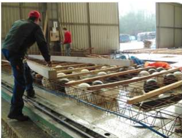
Fig. 8. Reinforcement spacers introduced in the self-compacting concrete. Gelissen Precast Factory (Holloweg)
