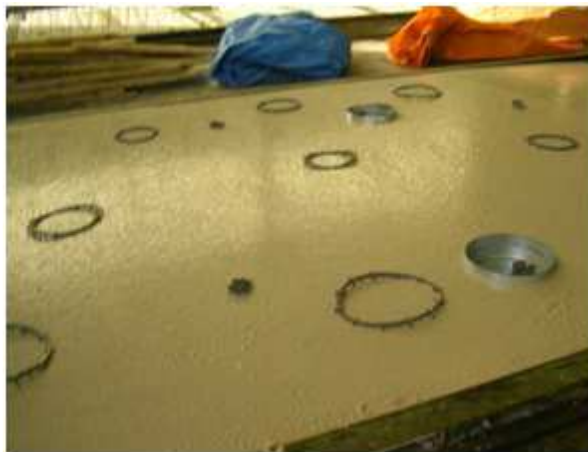
Fig. 8. Reinforcement spacers introduced in the self-compacting concrete. Gelissen Precast Factory (Holloweg)
