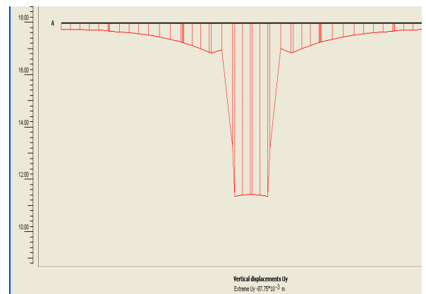
Fig. 9. Vertical displacements U_y at 17.96m – just below the foundation base
