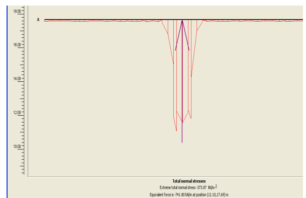
Fig. 10. Normal stress \sigma_y at 17.69m – just below the first reinforcement layer
