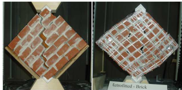
Fig. 5. Failure patterns of burned brick masonry wallettes (left) without retrofitting (right) with retrofitting (10)
