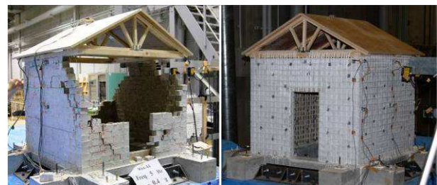
Fig. 2. Shaking table testing on non-retrofitted and retrofitted scale house model.
