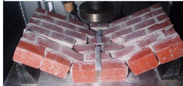
(a) Non-retrofitted wallette
