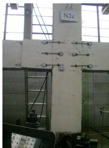
Fig. 5. Return to original shape after seismic-type loading
