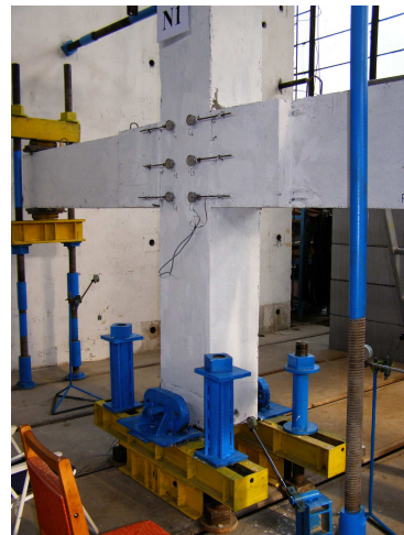
Fig. 3. Test set-up of hybrid and non-adherent hybrid joint specimens
