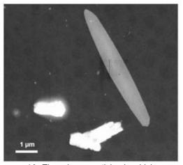
1A: Three large particles in which chemical elements are dominant: S, Ca, Na, O and Mg
