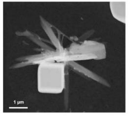
1C: Two types of particles, one particle with regular structure (sodium chloride crystal) and fibrous particles such as dominant chemical elements are: Ca. S. Na. O. Mg
